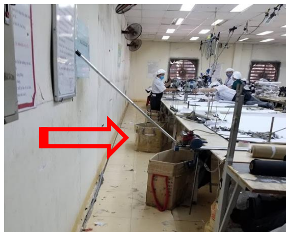
Figure 18: Activation Handle for Cutting Machine Protruding into Aisleway
