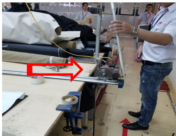
Figure 17: Unguarded Cutting Blade
