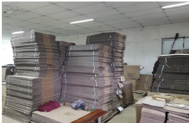
Figure 8: Excessive Storage of Combustible Packaging
