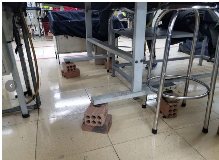
Figure 33: Worktable Propped-Up on Bricks
