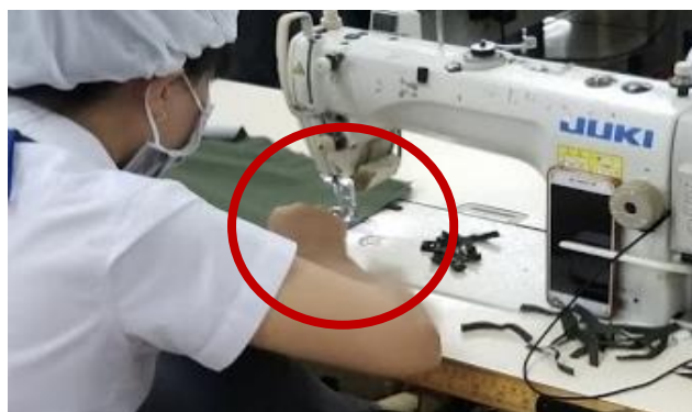
Figure 24: Lack of Guarding on Sewing Machines
